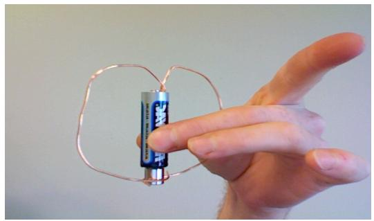
It really helps if the wire has its center of gravity either directly below the point it balances or close to underneath the point it balances on. If the center of gravity is too far off, then the center of gravity will try to shift to directly under the point the wire hangs from, often either introducing too much friction, or more likely pulling the top off of the battery.
