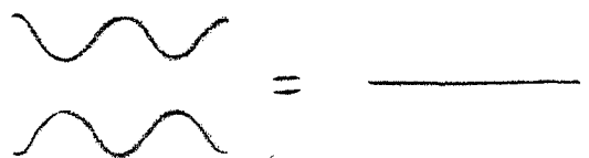
Figure 2 Destructive interference Combined, these waves cancel each other.
